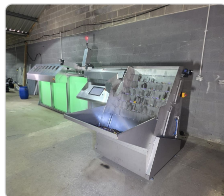
Sorted cells cascade to their chemistry fraction.
