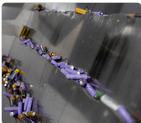
The step feeder settles mixed cells into an even flow.
