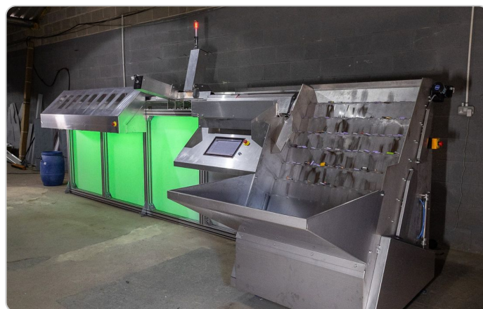
Hopper and step feeder, built in stainless for a recycling yard.
